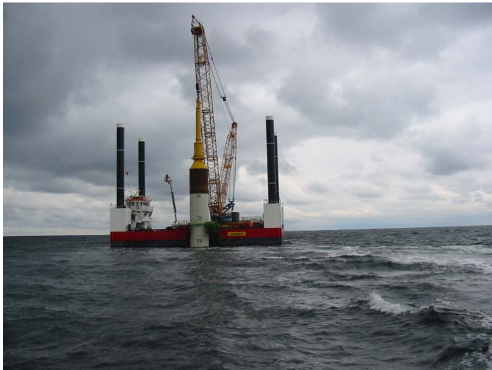
Figure 2: Shearlegs Samson with monopile and Jack-up Vagant (Samsø)
